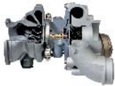
Waste Gate (WG) technology
